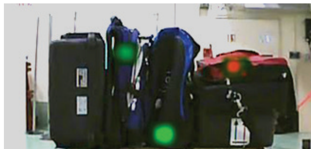
Figure 2 : Image of unattended luggages containing radioactive sources: two 241 Am sources (60 nSv/h and 161 nSv/h) and one 57 Co source (10nSv/h).
