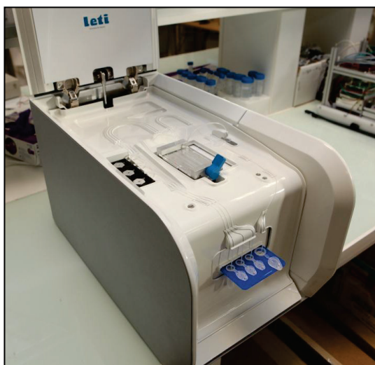
Figure 1: Prototype of a FlowPad instrument for automated sample preparation.
