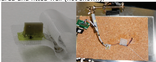
Figure 1: (left) The cuff electrode. (right) The 6-contact MCC recording electrode is located on the left of the worm while the stimulation ring electrode is on the right.
